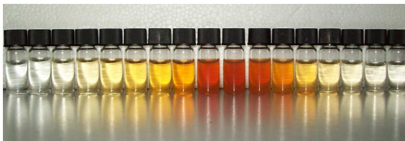
Fig. 3. Collected fractions of polyphosphate stabilized iron oxide nanoparticles after A4F-SAXS measurement. The fractionation time increases from left to right in sequence with the increasing radii of the particles.
